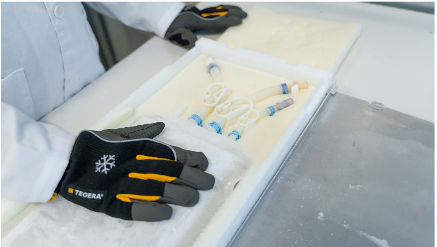
Figure 5: RoSS® shells significantly reduce product loss when handling single-use bags in biopharmaceutical processes
