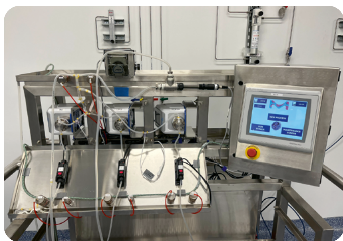
Figure 1. Automated process development skid enables controlled and efficient manufacturing of LNPs.
